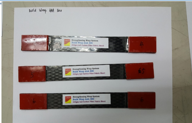
Specimen Sample: CFRP Wrap for 300gsm/m2
